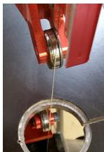
The Pégas® guiding system is required whilst using Pégas® scroll bandsaw blades. The blade will be guided accurately for high-performance, sustainable sawing results.
